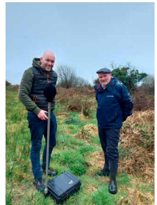
A noise monitor being installed
